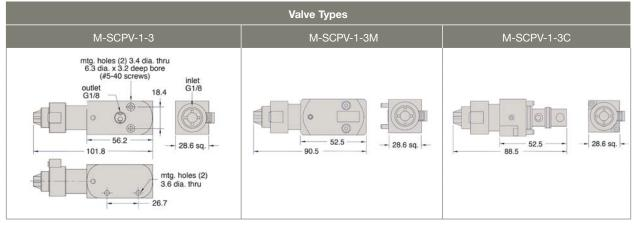
Utilizing the industry's most robust and powerful linear actuator, the highflow stepper-controlled proportional valve outperforms the competition in performance and durability.
